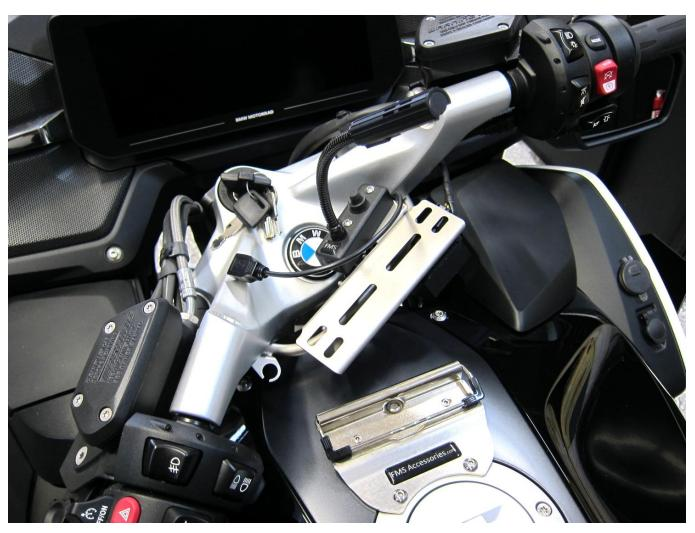
The FMS Cell Phone Power Converter is designed to provide power to your cell phone or charger base utilizing the map light power plug under the RH handlebar, rather than connecting to the USB / Voltmeter socket in the fairing.
